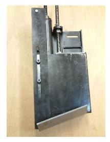
**Creating Safety Edge Slopes less than 30°.** In some cases, say for example because of rolling patterns that tend to push out the asphalt thereby increasing the slope angle that was initially created by the shoe, the operator my wish to create a slightly flatter angle so that the final result will tie in with a 30° slope.
